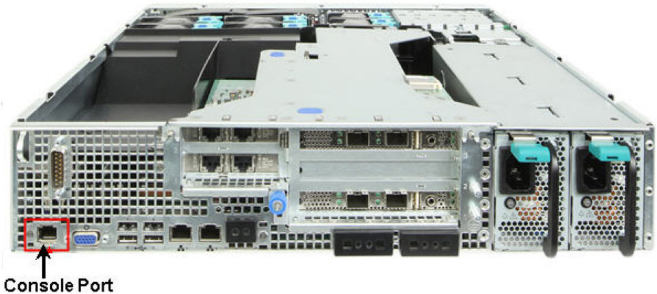
FIGURE 2 SZ300 Location of console port
